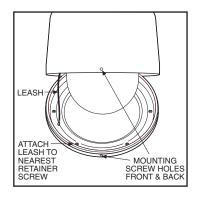
b. Attach the back box trim leash to the lower dome. Use retainer screw (nearest to a mounting screw) inside lower dome.
